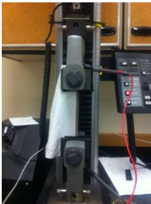
Figure 3. Experimental setup: sample mounted in Instron with DMM leads attached (top and bottom)
