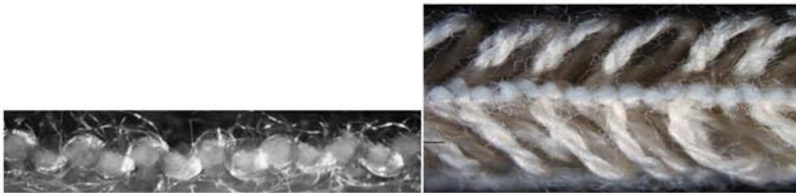
Figure 2. Cross-sectional views of terry and plain fabrics (a) Plain Fabric (b) Terry fabric
