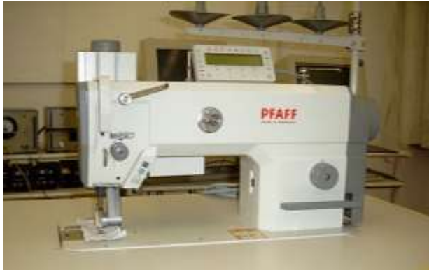
Figure 2. A special high-speed Pfaff 1427 sewing machine
