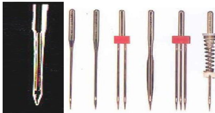
Fig 3. Cryogenically Treated sewing & various types of sewing needles
