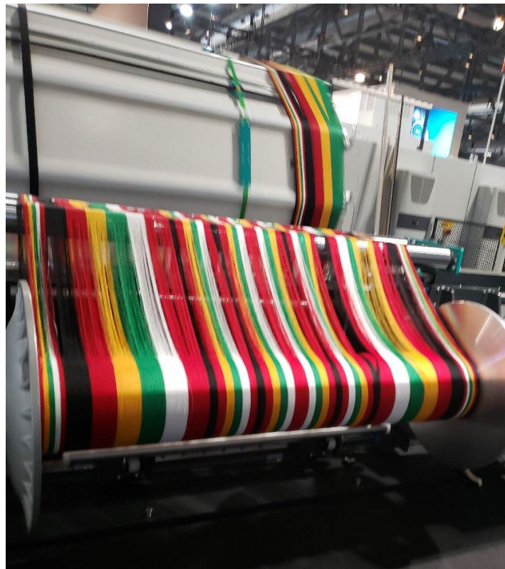
Figure 1. Multi-Matic® 32 Compact Sample Waring Machine
