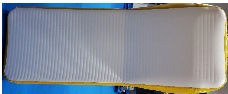
Figure 9. Inflated Boat from Variable Height Distance Fabric
