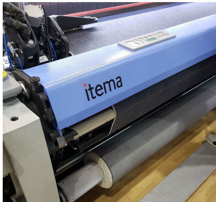
Figure 6. R9500EVO Machine Equipped the iSAVER® forming Denim Fabric
