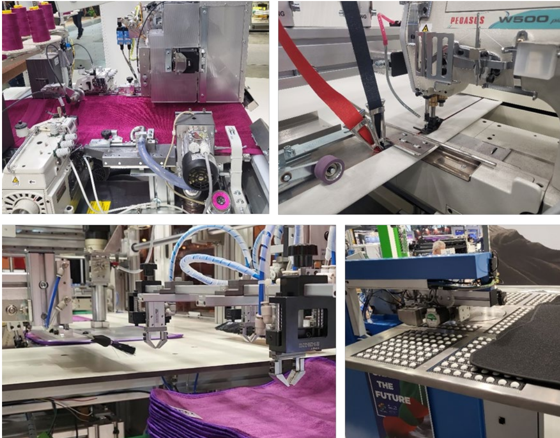
Figure 6. Automated sewing for towels by Schmale Durate (top left) and TPET (bottom left), bed sheets by Texpa (top right), and mats by Rimac (bottom right)
