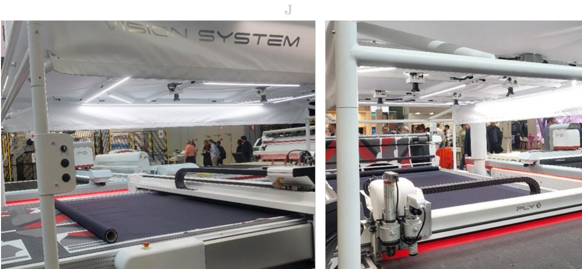
Figure 4. Morgan Tecnica Vision System (left) with multiple low-mounted cameras (right)
