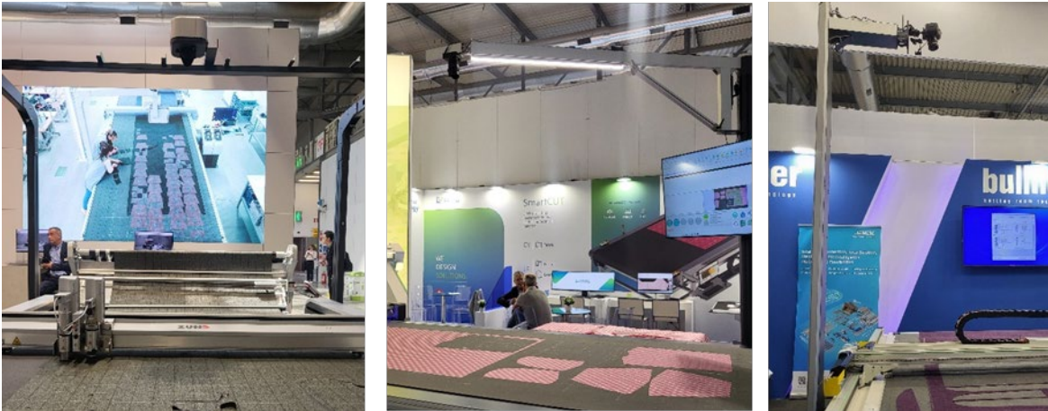
Figure 3. High-mounted cameras for fabric pattern alignment by Zund (left), Lakeview Technology (middle), and Bullmer (right)
