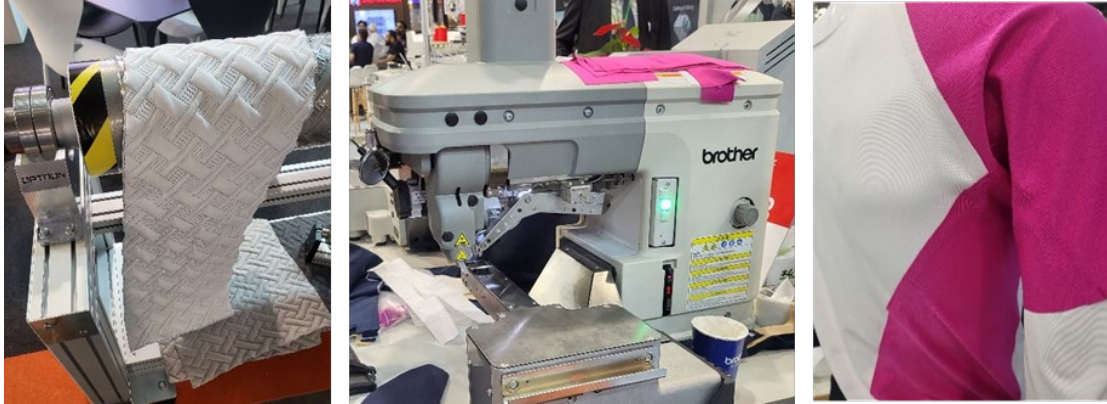
Figure 11. Alternative sewing technologies: welded quilting by Optron (left), bonded seaming by Brother (middle) and the resulting seams (right)
