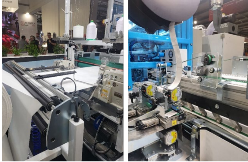
Figure 7. Fully automated pillowcase maker by Automatex: feeding and seaming (left) and labeling (right)
