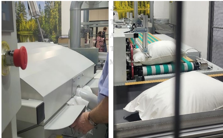
Figure 8. Automated pillow maker by ACG Kinna Automatic: filling (left) and closing (right)
