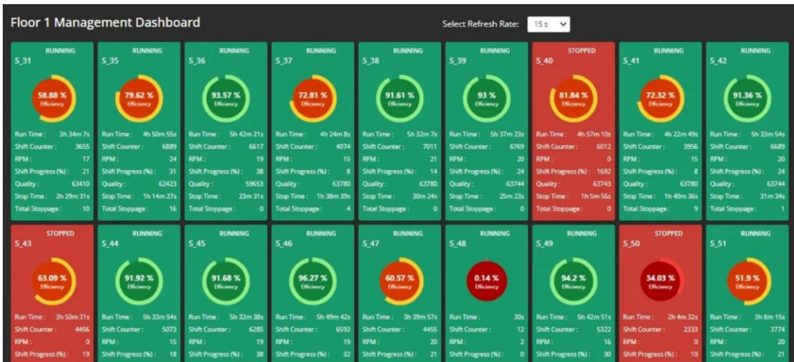
Image 2: Machine Floor Tile View Dashboard with production parameters (XdotO)
