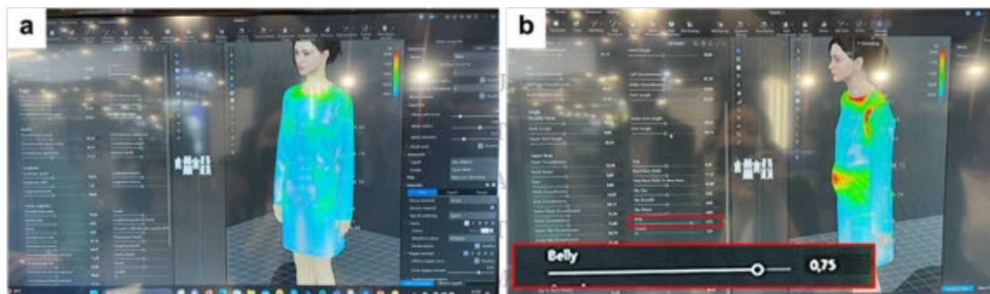
Figure 7. Fitting Evaluation and Avatar Customization in Style 3D Design Software. A demonstration of advanced features of Style 3D, showcasing (a) simultaneous adjustments of avatar body sizes, facial expressions, poses, and animations for fit evaluation, and (b) simulation of a pregnant condition by modifying the belly size. Images captured from a demonstration at ITMA 2023 by © Style3D with permission.
