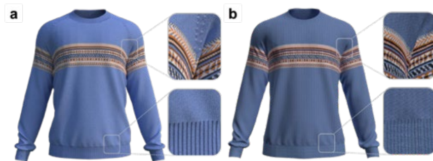
Figure 8. Comparing Yarn Simulation for a Fully Fashioned Style Using CREATE DESIGN and Cut & Sew 3D Garment Simulation Using Scanned Texture and Repeats. (a) High-fidelity yarn simulation showcasing stitch decreases and fully fashioned marks in detail, (b) 3D garment simulation with a lack of stitch decreases and fully fashioned marks. Images were captured from a document provided by © KM.ON.
