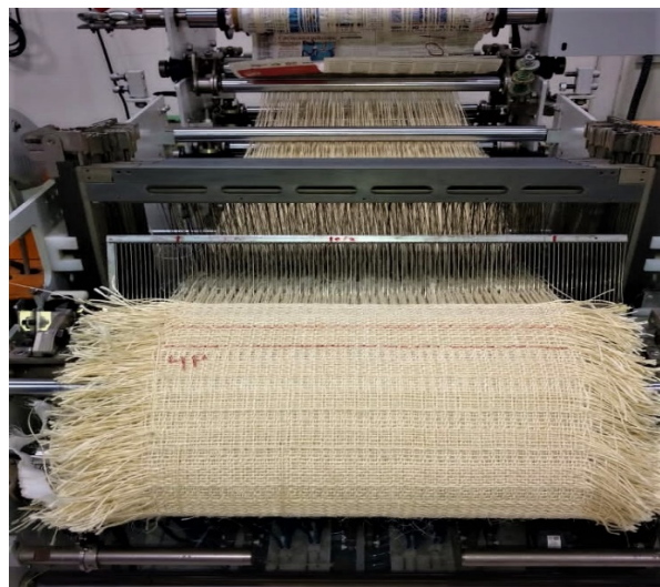
Figure 3. Customized rapier weaving machine
