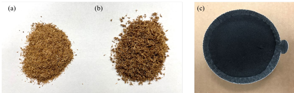
Figure 1. Images of short CFs with an average length of (a) ~ 1 mm, (b) ~ 2 mm and (c) MRP.
