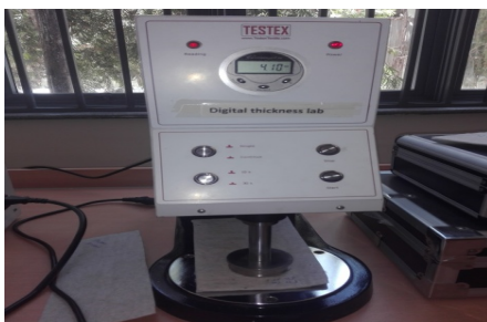
Figure 2.1. Digital thickness tester machine
