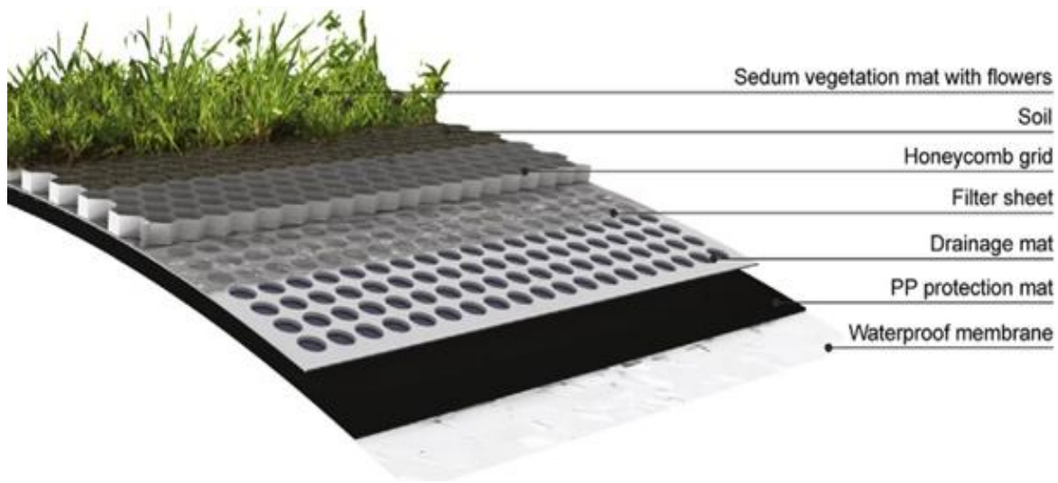
Figure 6: Green textile roofs multilayered structure [50]
