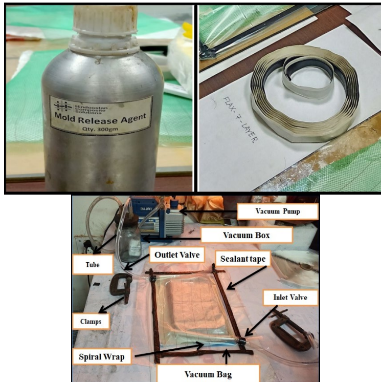
Figure 1. (a) Mold release agent, (b) Tacky tape, and (c) VARTM Setup
