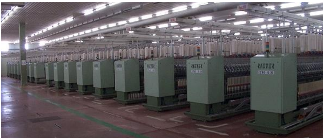
Figure 2. A view from ring spinning machines on which the roving bobbins and cops on the spindles are located.
