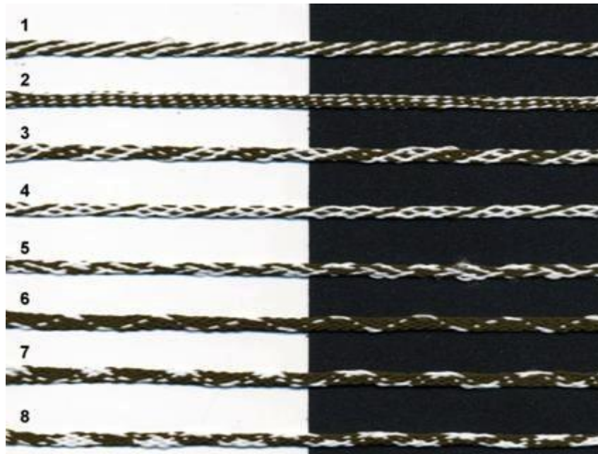
Figure 9. 1x1 Two-color Patterns: 1. Diagonal Stripe 2. Pinstripe 3. Small Chain-like Pattern 4. Large Chain-like Pattern 5. Twisted Pattern 6. Thin Diamond 7. Thicker Diamond 8. Thickest Diamond (Color Block)
