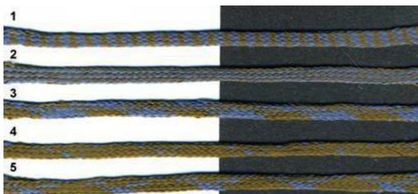
Figure 6. 2x2 Two-Color Braid Patterns: 1. Horizontal Zig-Zag Stripe 2. Pinstripe 3. Argyle 4. Thin Diamond 5. Thick Diamond
