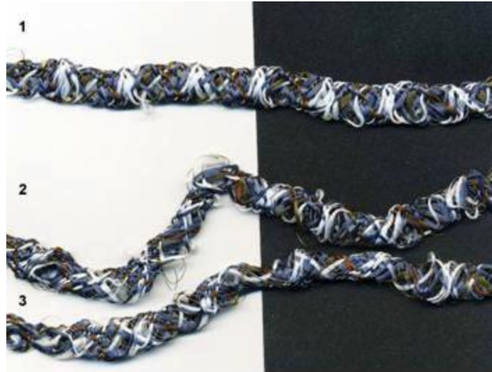
Figure 16. 2x2 Wire Studies: 1. 12 ppi Four Wires, Opposing Directions 2. 12 ppi Six Wires, Opposing Directions 3. 12 ppi Eight Wires, Opposing Directions
