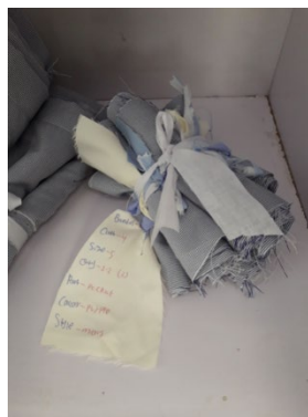
Figure 2: Manual bundle ticketing
