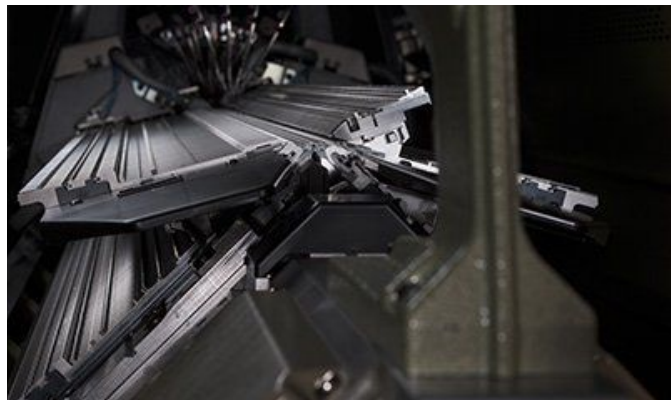
Fig 8. MACH2XS and MACH2X present a technological breakthrough in modern computerized flat knitting, in its 4-needlebed configuration, featuring 2 extra beds on top of a conventional V-bed. © Shima Seiki
