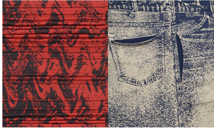
Fig 7. i-Plating offers inverse-plating capability in which different yarns can be shown alternately on the fabric surface for a jacquard-like effect in plain jersey stitch. © Shima Seiki
