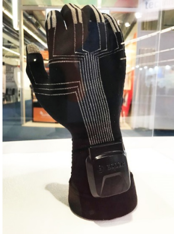
Fig 17. Knitted augmented and virtual reality sensor glove. © Stoll
