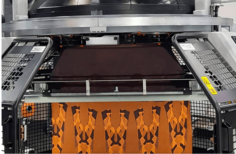
Fig 26. Mayer & Cie.’s double jacquard OVJA 1.1 EETT machine knitting shoes. © Mayer & Cie.
