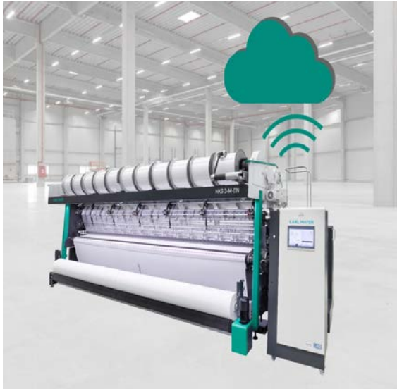
Fig 27 and 28. The HKS 3-M-ON is the first three-bar HKS model with electronic guide bar control that allows immediate pattern changes © Karl Mayer
