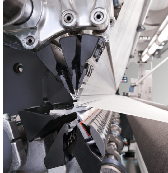
Fig 27 and 28. The HKS 3-M-ON is the first three-bar HKS model with electronic guide bar control that allows immediate pattern changes © Karl Mayer
