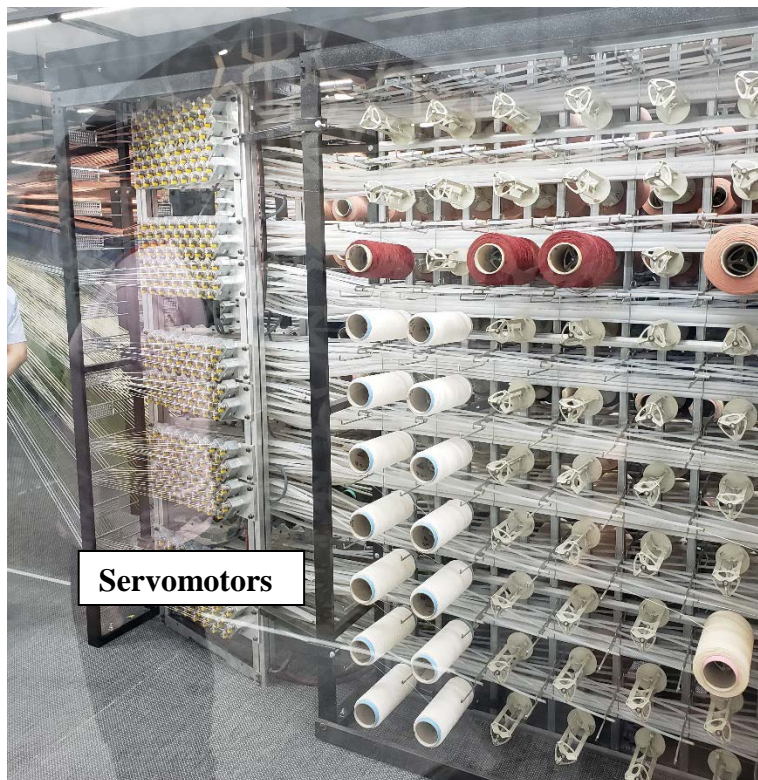
Figure 5. VANDEWIELE’s Fast Creel of rotating packages and servomotors
