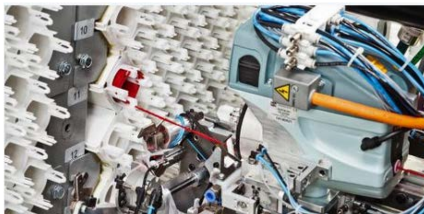
Figure 3. VANDEWIELE’s Smart Creel Robot winding a red yarn onto a cell (Source: https://www.vandewiele.be/en/activities/smart-creel , retrieved July 21, 2019)
