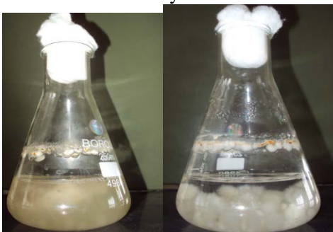
Figure 3. AATCC 30- Broth Dilution Test
