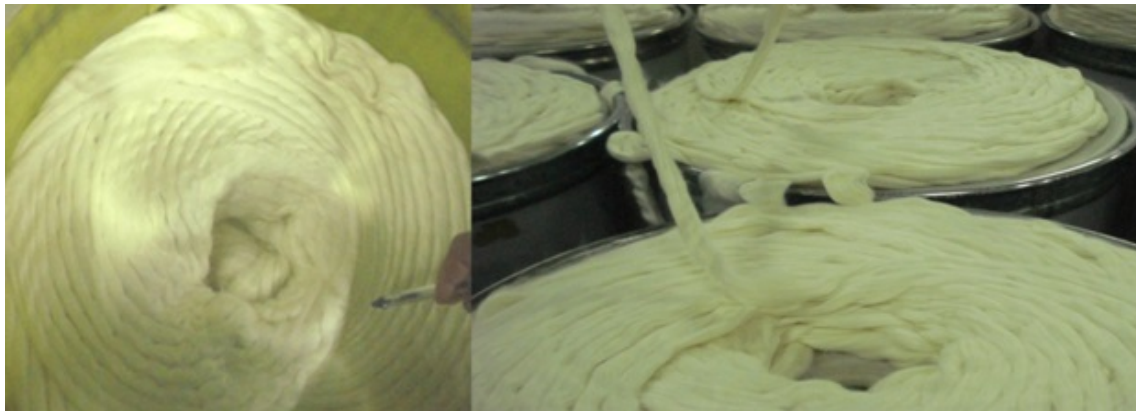
Figure 5. Flattened sliver coils at the end of the batch at speedframe creel zone.
