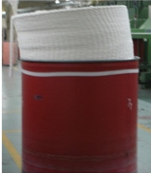
Figure 4. Stored combed sliver touching side wall due to spring buckling in an older can
