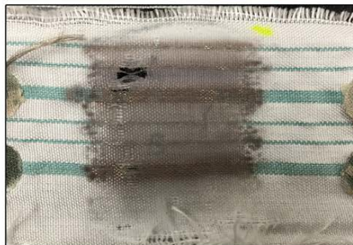
Figure 7. Wyzenbeek Test Sample Photos: Network A is top trace and Network B is bottom trace in pictured test sample. The onset of failure occurred at different cycles of abrasion testing. A possible explanation for the variation in the number of abrasion cycles is based on the formation factors, e-yarn type and number of e- yarns in the trace.
