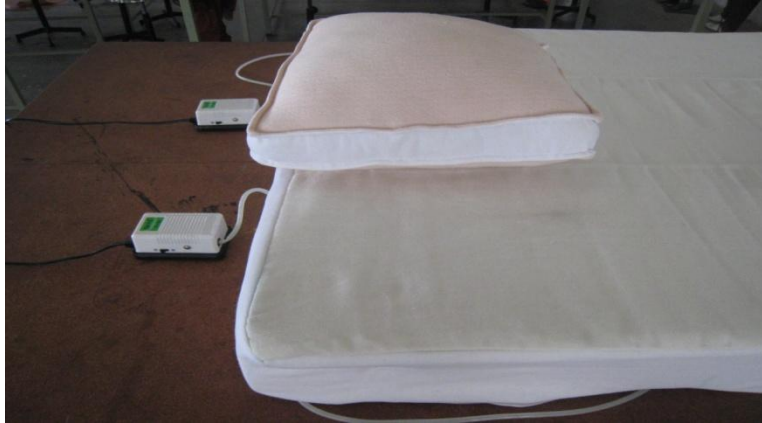
FIGURE 9. ILLUSTRATION OF MULTILAYERED BED WITH AIR CIRCULATION MEASURING KID
