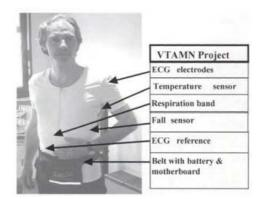
Figure 11. VTAMN prototype (Dittmar et al., 2004)
