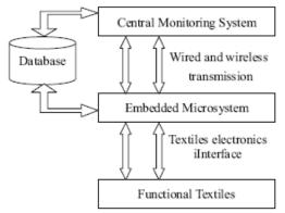
Figure 9. The architectural level of a smart sport underwear system (Liu & Sun, 2006)
