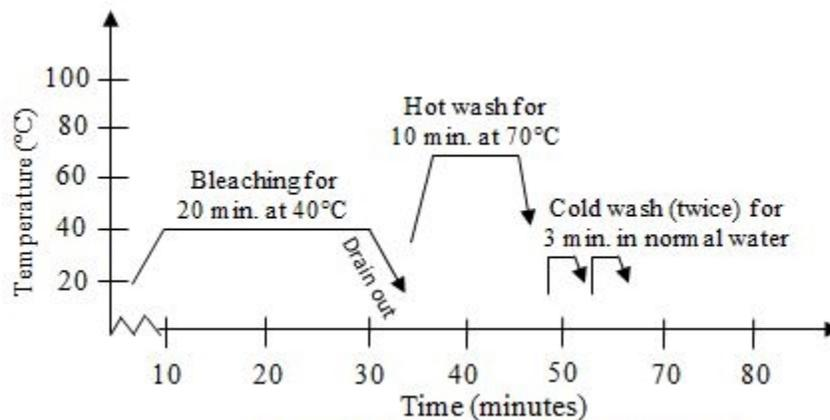
**Figure 2: Bleach washing process curve**
