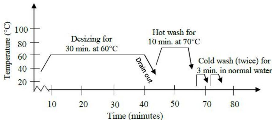
Figure 1: Desizing process curve
